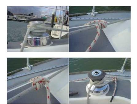
You will almost certainly find that the normal rolling hitch where the rope is passed twice round the loaded rope does not work. It is normally necessary to pass the rope around the loaded one 4 or 5 times to achieve sufficient grip.
