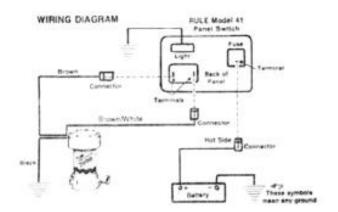
The plain brown lead should be connected to the automatic position on the switch and the brown/red lead should be connected to the manual position.
